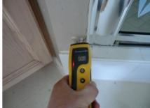
Besides we reiterated the bath ventilation enforcement, it is better to swipe the water on the wall into the pan after shower in order to reduce the chance moisture intrusion to the wall. Grouting & caulking should be a regular maintenance in every summer or fall.
